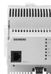
Side-connection extension module PXX.. for modular series PXC..D
