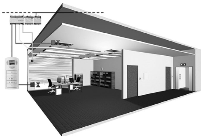
Integrated operation of HVAC, lighting and blinds with Desigo RXC
